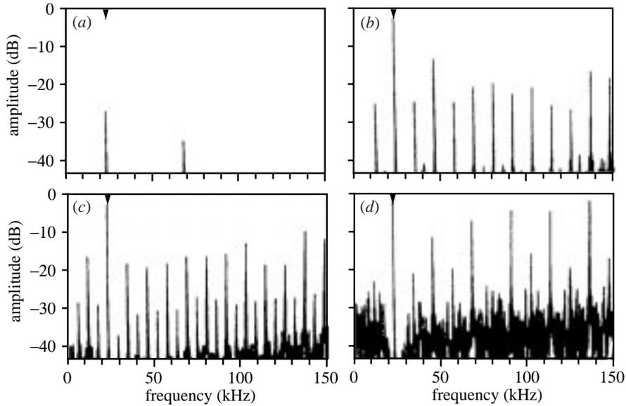
Figure 20. Power spectra of cavitation noise taken at a driving frequency of  $f_0 = 23$  kHz, marked in the figures by a small upside down triangle. The driving pressure was increased from one graph to the next, giving first a periodic anharmonic signal (a), then subharmonic motion with lines at multiples of  $\frac{1}{2}f_0$  (period-2 motion) (b), then period-4 motion with lines at multiples of  $\frac{1}{4}f_0$  (c), and finally a broadband spectrum indicative of chaotic behaviour (d).
