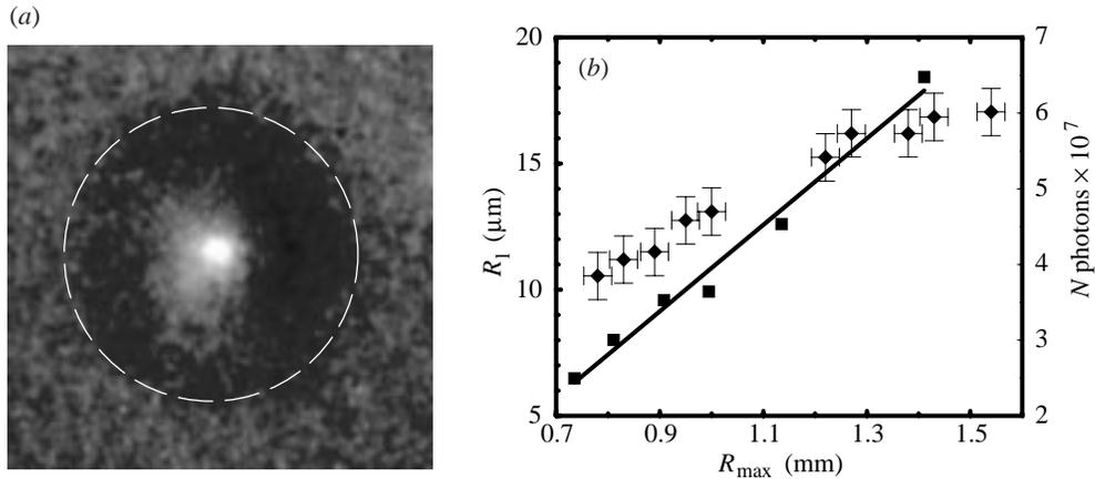
Figure 14. SCBL. (a) Light emission from a laser-generated bubble upon first collapse. Superimposed on the image is an outline of the maximum bubble size before collapse. (b) Radius  $R_1$  of the emission spot (diamonds) and number  $N$  of photons emitted (squares) as a function of the maximum radius of the bubble.
