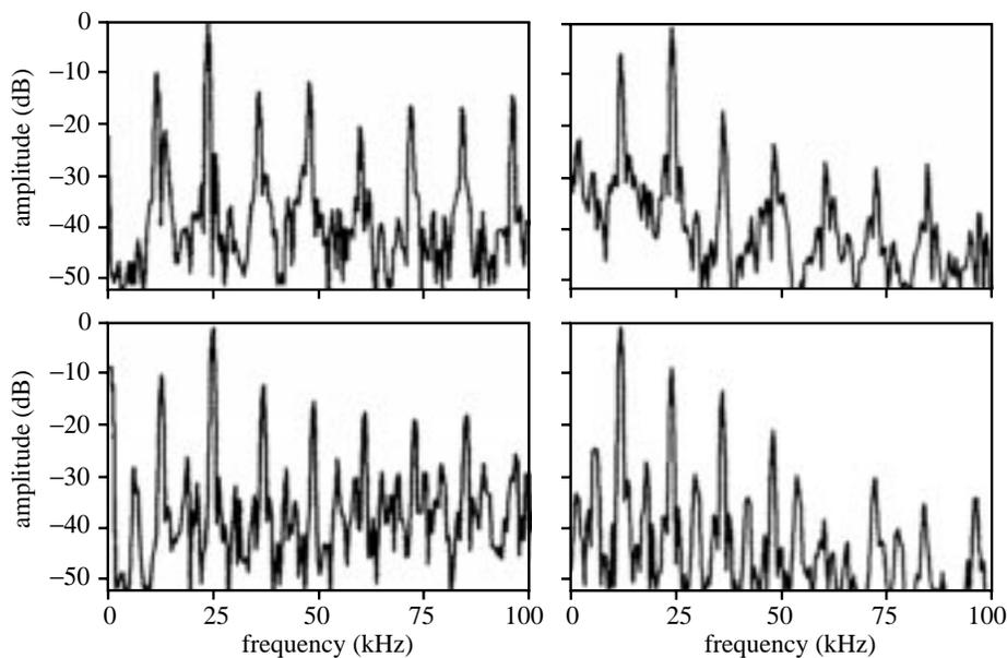
Figure 19. Comparison of the acoustic spectra of cavitation noise (left) and the power spectra of the light transmission signal (right) obtained with the arrangement of figure 18 for two different driving pressures at frequency  $f_0 = 23.1$  kHz: (top row) subharmonic response giving multiples of  $\frac{1}{2}f_0$ ; (bottom row) response giving multiples of  $\frac{1}{4}f_0$ .
