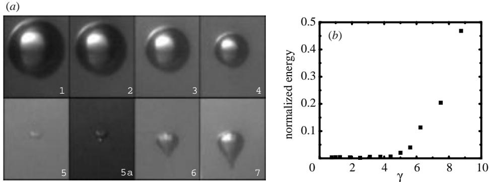
Figure 15. Luminescence of an asymmetrically collapsing laser-generated bubble. (a) Photographic sequence indicating the maximum bubble size and the location of the light-emitting spot with  $\gamma = 4.7$ . Frame 5a is a copy of frame 5 with an image of the light-emitting spot superimposed. (b) Dependence of light intensity, normalized to the emission at spherical collapse, on the distance parameter  $\gamma$ .
