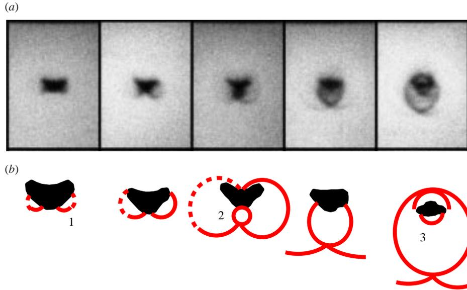
Figure 10. Scenario of asymmetric bubble collapse with indication of the different shock waves emitted. The size of the individual frames is  $2.0 \times 1.4 \text{ mm}^2$  and the asymmetry parameter is  $\gamma = 2.7$ .
