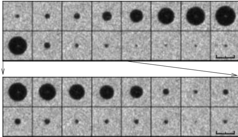
Figure 5. Photographic series of a trapped sonoluminescing bubble driven at 21.4 kHz. The top row presents the bubble dynamics at an interframe time of *ca.* 2.5  $\mu$ s. The bottom row shows the bubble collapse with five-fold temporal resolution (500 ns interframe time). The scale of the image is indicated by the ruler (100  $\mu$ m).
