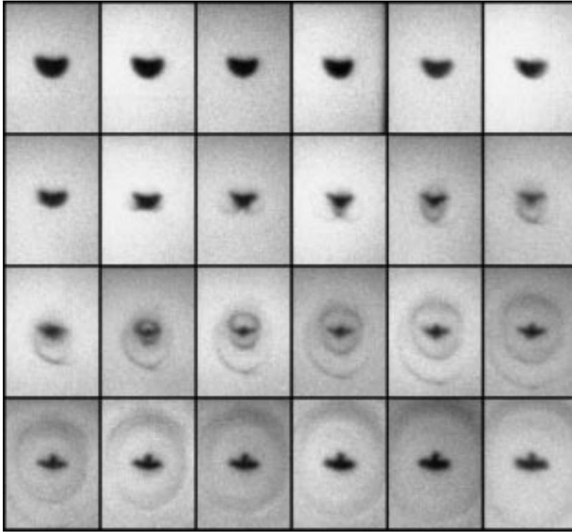
Figure 11. Collapse of a laser-generated cavitation bubble near a solid boundary (out of view below each frame) taken at 20.8 million frames per second. Relative distance to the boundary is  $\gamma = 2.4$ . Three shock waves are emitted: the jet torus shock wave (frames 8–10), the tip bubble shock wave (frame 10 onwards) and the main bubble shock wave (frame 13 onwards). The frames are counted from left to right and from top to bottom. The frame size is  $2.0 \times 1.4$  mm.
